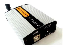
Sim900a GSM/GPRS USB Modem, Featuring an industry-standard interface, the SIM900A delivers GSM/GPRS 900/1800MHz performance for SMS, Data, and Fax in a small form factor and with low power consumption, With Aluminum enclosure to minimize noise.
